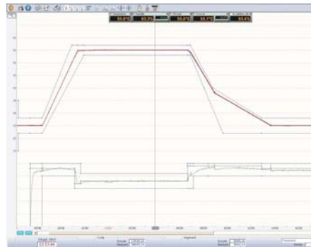
Example of an IEC 60068-2-30 test
