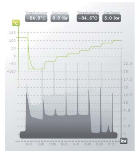
This standard test cycle clearly shows the energy saved with the "Energy saving" cycle (dark grey curve) compared with a cycle without this mode (light grey curve). Electrical consumptions are displayed instantly.
