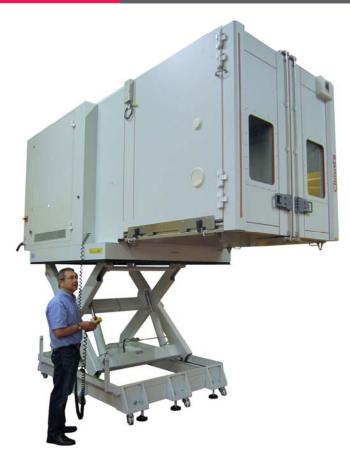
Mobile on two axes and assisted for its vertical moves, this hot – cold- humidity chamber enables to test wide products in vibration and temperature combined conditions.
