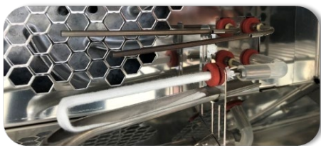
Control sensor + independent safety sensor + Psychrometric sensor
